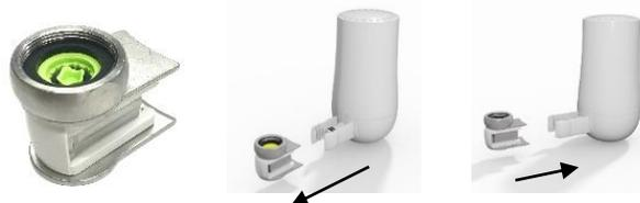
4. Unpackage replacement faucet filter and slide it onto the connector until it locks into place.
